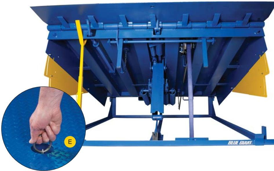
The Blue Giant U-Series mechanical dock leveler is easy to use: simply pull the release chain and let the heavy duty main lift springs go into action. The deck rises up and the lip extends smoothly to the locked position. Then 'walk' the deck down to the truck bed and begin loading or unloading.
